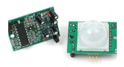
Figure 3. PIR motion Sensor
