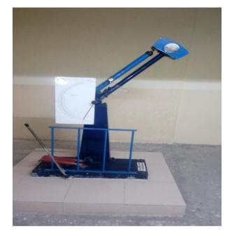
Fig. 3 Experimental set up of charpy impact testing.
