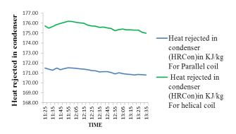
**Chart -7**: Heat rejected in condenser For parallel Vs Helical coil condenser
