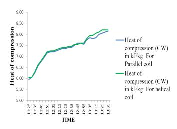
Chart -3: Compressor work For parallel Vs Helical coil condenser
