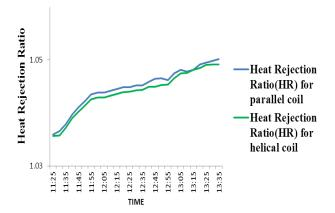
Chart -9: Heat rejection ratio For parallel Vs Helical coil condenser
