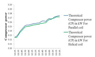
Chart -5: Theoretical power For parallel Vs Helical coil condenser
