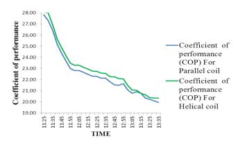
Chart -6: COP For parallel Vs Helical coil condenser
