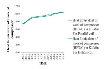
**Chart -4**: Equivalent work For parallel Vs Helical coil condenser
