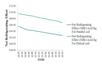
Chart -1: NRE For parallel Vs Helical coil condenser
