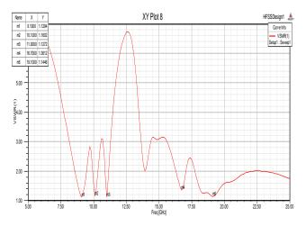
Fig 7: VSWR plot after last iteration
