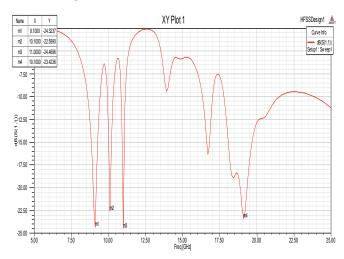
Fig 6: Return loss after last iteration
