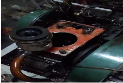
Fig: 3.4 .inside part of a cylinder head when combustion chamber is changing
