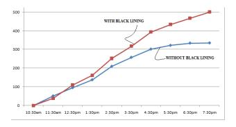
Graph No 5: Comparison of Single slope single basin solar still with and without black coating
