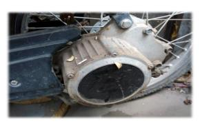
Fig-6: Motor Coupled with rear wheel
