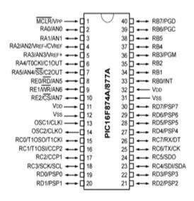
Fig. 2. Pin configuration of the PIC 16F877A microcontroller
