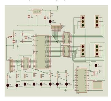
Fig. 3. Block diagram of the circuit designed by Proteus software. The handheld portable controller hardware is is disposed at left while the traffic master controller implementation is shown at the right.
