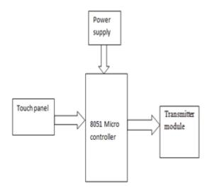
Fig -2: Transmission Section
