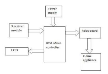
Fig -3: Receiver Section
