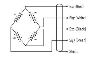
Fig. 3(a). Typical load cell diagram.
