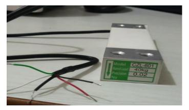
Fig. 3(b). Single point load cell.
