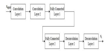
Fig – 2: Architecture of CNN used in music source separation and recognition
