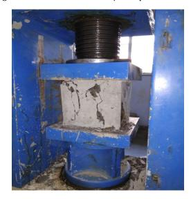
**Fig -1:** Compressive strength Test
