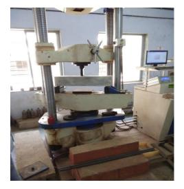
Fig -2: Flexural strength Test
