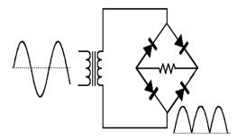
**Fig -1**: A bridge rectifier
