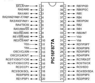
Fig -4: pin configuration and description of PIC16F877A
