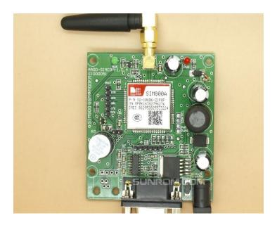
Fig (3) GSM Module
