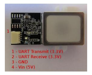
Fig (2) Fingerprint Module
