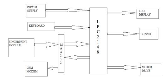
Fig (1) Block Diagram of LPC2148
