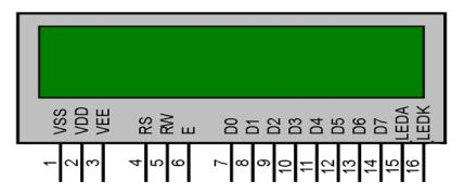
Fig (4) LCD Display
