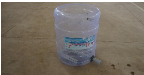
Fig.6 (a): Filtration unit draining pipe setup (Front view)
