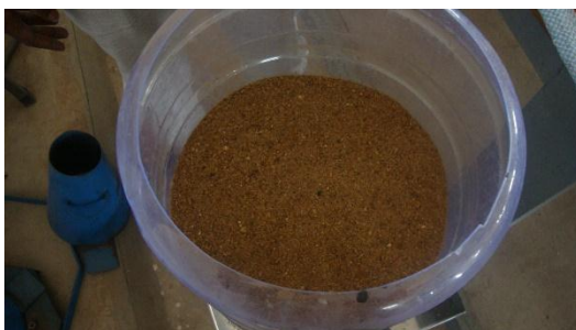
Fig.8: Fill the Fine aggregate in filtration unit
