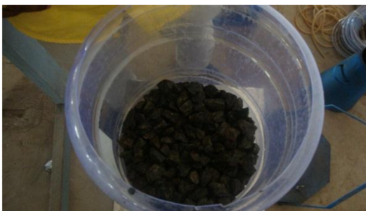
Fig.7: Fill the Coarse aggregate in filtration unit
