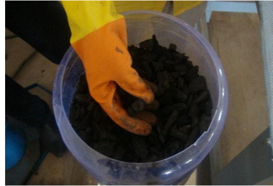
Fig.9: Fill the Activated charcoal in filtration unit
