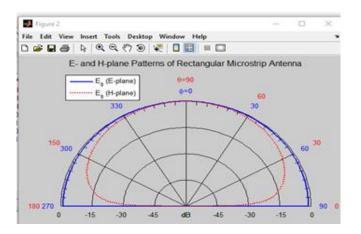
Fig-2:radiation pattren of rectangular patch
