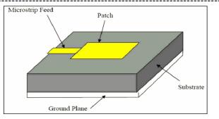
Fig-1: Microstrip patch antenna
