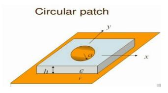
Fig-3:circular patch antenna
