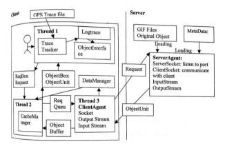
Figure 4.2: Main Components and Architecture of Mobile System
