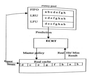
Figure 5.1: Design of ECRT: Voting Mechanism
