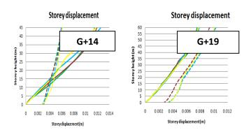
Fig 5 Maximum storey displacement with storey height
