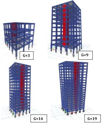
Fig -2: 3D view of base isolated structure with different heights
