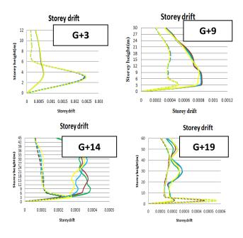
Fig 6 Maximum storey drift with storey height
