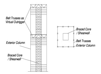
Fig.1 Belt Truss as Virtual Outrigger
