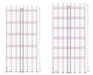
Fig.4 Belt Truss at 5 storey Interval Model-II
