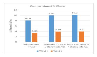
Fig.3 Comparison of Stiffness in Wind X and Y Directions for tall buildings with and without Belt truss
