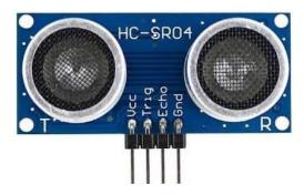
The Ultrasonic Sensor sends frequency sound pulse of high range and then measures the time taken by the sound to reflect back. The front side of the sensor has 2 openings. Ultrasonic wave is transmitted by one opening and received by the other. The distance of the object is calculated by the difference between sending and receiving sound pulse. Here, HC-SR04 ultrasonic sensor is used which provides noncontact measurement function of 2cm to 400cm.
