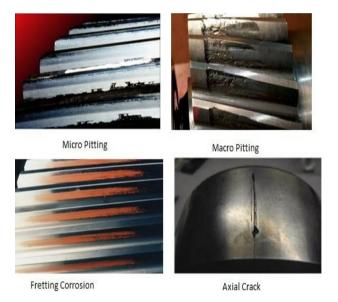
Figure.3 Failure due to load
