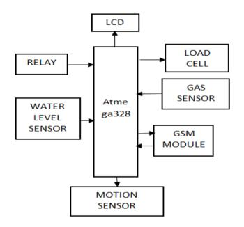
Fig. 1: BLOCK DIAGRAM OF LPG LEAKAGE DETECTION AND PREVENTION SYSTEM WITH GSM ALERT
