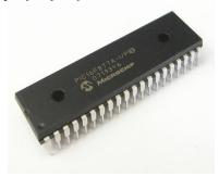
Fig. PIC Microcontroller 16F877A
