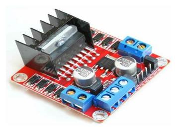
Fig -4: Motor Driver ST L298N (5 Amps Peak)
