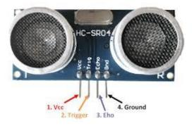
Fig -6: Ultrasonic Sensor
