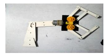
Fig -2: Partial Attachment of robotic arm
