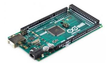
Fig -10: Arduino Mega 2560 R3 Micro Controller
