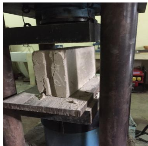
Figure - 2: Failure mode of concrete block after loading.
