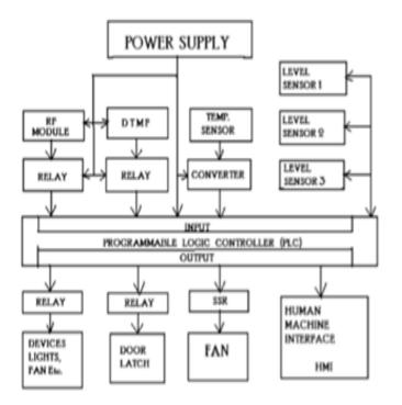
Fig -1: Existing Block Diagram
