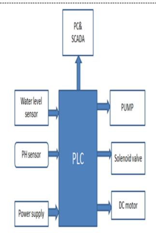
Fig -1: Block diagram of Recycling Process
