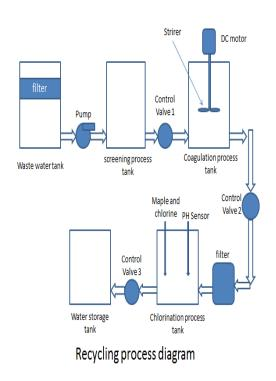
Fig -2: Recycling Process Diagram
