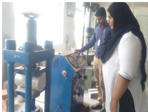
Fig -3: Split Tensile Strength Test
