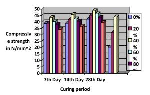
Fig 1. Compressive strength of geopolymer concrete with replacement of fine aggregates by iron ore tailings
