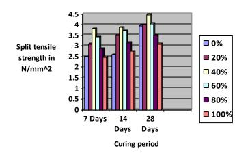
Fig 1.2 Split tensile strength of geopolymer concrete with replacement of fine aggregates by iron ore tailings.
