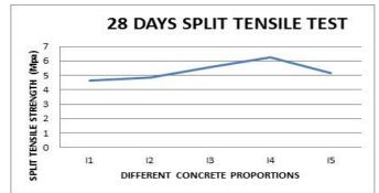
Figure 9: 28 Days Split Tensile Test for Different Concrete Mix
