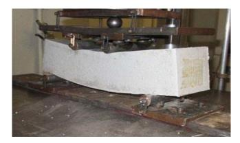
Figure 4: Flexural strength of beams
