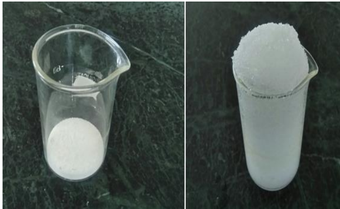
Fig-1 : Swelling characteristics of SAP used (Before and after Swell)
