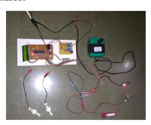
This is result of system. When low level and high level of water tank is sensed by low level and high level sensor respectively, then hydraulic pump becomes automatically on and off according to condition and the message is displayed on LCD display. Similarly fire is detected by fire sensor and buzzer remains on continuously. When gas is detected by LPG Gas sensor, buzzer is on but it will not remains continuously on.
