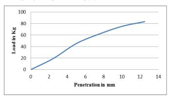
Fig.1. Results of CBR test on Red soil without Geo-grid
