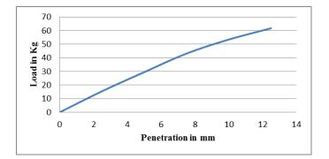
Fig.3.Results of CBR test on black cotton soil without Geo-grid
