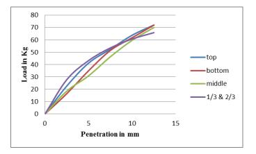
Fig.4.Results of test on black cotton soil with Geo-grid
