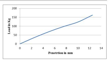
Fig.7. Results of CBR test on alluvial soil without Geogrid
