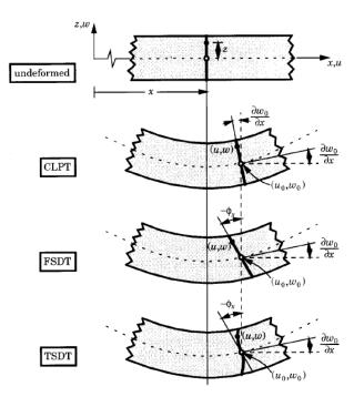
Fig-3: Transverse shear deformation of a plane according to various plate theories
