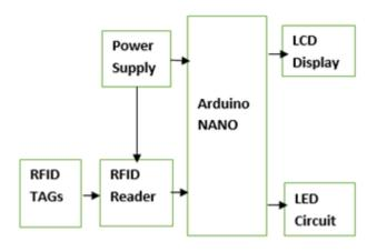
Figure 1: Block Diagram of Proposed System
