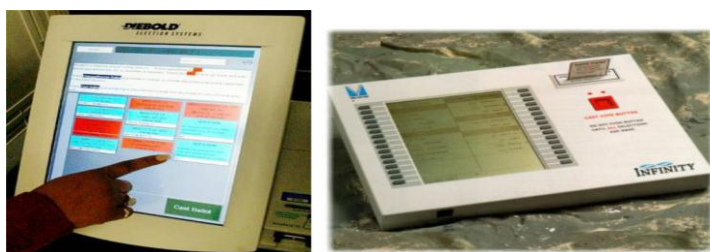
Figure 2.2: Touch screen & other electronic voting machine
