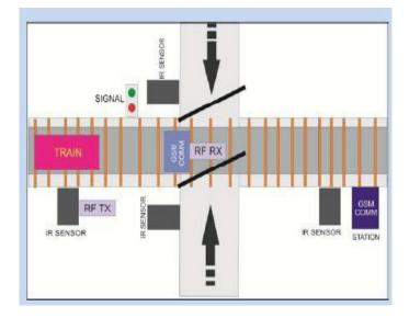
Figure 1.3: Automated Railway Crossing System [10]
