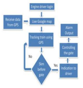
Figure 2.12: System using GPS and GSM [8]
