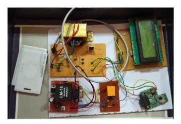
Fig-4: Complete hardware structure of the system without  $$\operatorname{PC}$$
