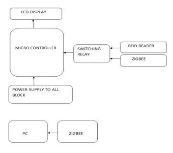
Fig-2: Block diagram of Students Smart Card
