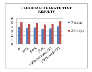
Fig-6: comparisons of flexural strength
