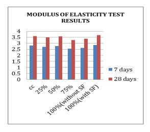
Fig-5:comparison of modulus of elasticity test
