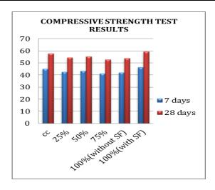
Fig-3:comparisons of compressive strength
