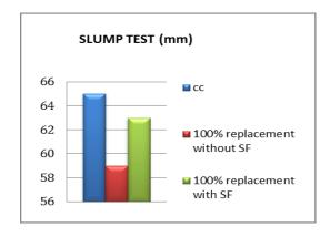
Fig.2:slump test results
