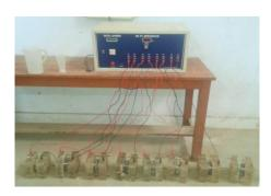
Fig-10: RCPT Setup
