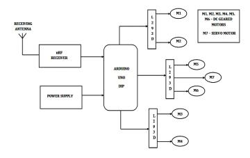
Figure 5: Block Diagram of Receiver
