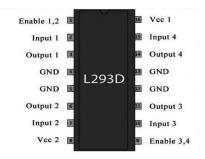
Figure 6: Pin Diagram of L293D IC
