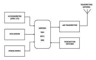
Figure 1: Block Diagram of Transmitter
