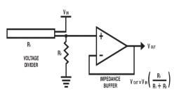
Figure 4: Circuit Diagram of Flex Sensor
