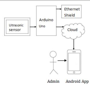
Fig-1: System Architecture
