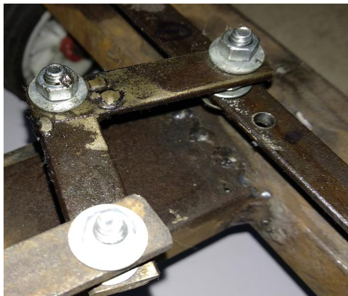
Fig -2: L type Link that moves Ackerman Steering
