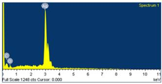
Spectrum processing: Peak possibly omitted: 7.540 keV Processing option: All elements analyzed (Normalised) Number of iterations = 2 Standard: C CaCO3 1-Jun-1999 12:00 AM O SiO2 1-Jun-1999 12:00 AM Ag Ag 1-Jun-1999 12:00 AM
