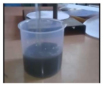
The solution, which was subjected to vigorous agitation, turned yellow immediately and then black. The obtained solution is centrifugated and silver nanopowder will be collected at the bottom of the test tube as shown in the figure.
