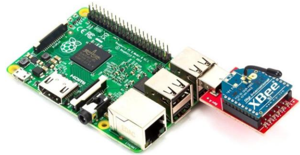
Fig-8: XBEE CONFIGURED WITH RASPBERRY PI
