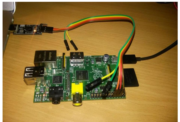
Fig-9 : RASPBERRY PI CONNECTS WITH UART
