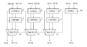
Fig 3(b). carry select adder with BEC
