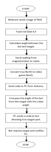
Fig 2: The flowchart clearly shows a step by step functioning of the entire system.
