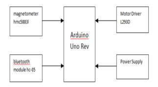
Fig 3: Figure illustrates the major blocks of operating hardware components.
