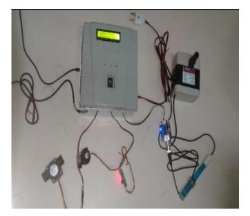
FIG 3. SYSTEM OUTPUT ON IOT BESED WATER MONITORING SYSTEM
