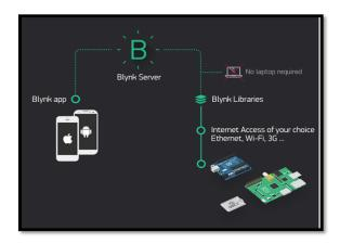
FIG 1.ARCHITECTURE OF BLYNK SOFTWARE
