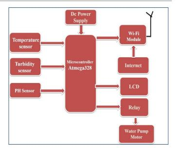
FIG 4. BLOCK DIAGRAM OF WATER MONITORING SYSTEM
