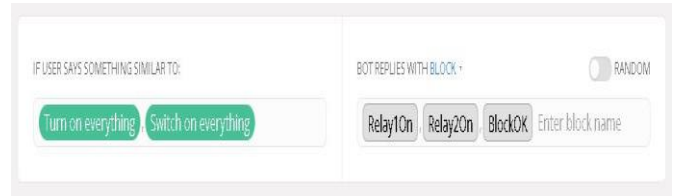
Fig -2: An AI rule on Chatfuel to turn on both the relays.
