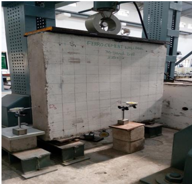
Fig-6: Test Setup for Ferro-Cement M-Sand Infill Wall Panel.
