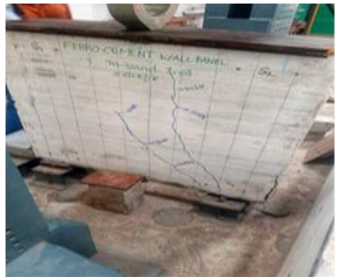
Fig-8: Crack Pattern of M-Sand Infill Wall Panel
