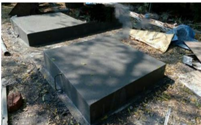
Fig-4: The Infill Materials Such as Red Soil in Wall Panel-P1, M-Sand in Wall Panel -P2.
