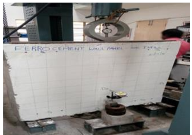
Fig-5: Test Setup for Ferro-Cement Red Soil Infill Wall Panel
