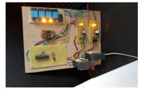
Fig 5: Valve Controlling Node
