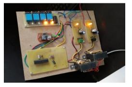
Fig 9: Valve Controlling Node
